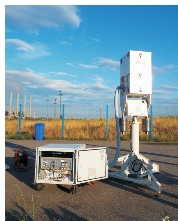
Lidar set-up for scanning of the plume
